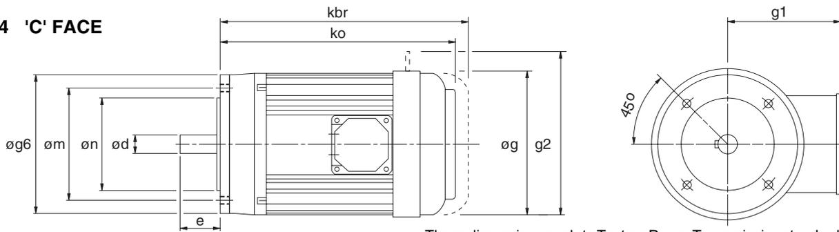
These dimensions apply to Textron Power Transmission standard motors
