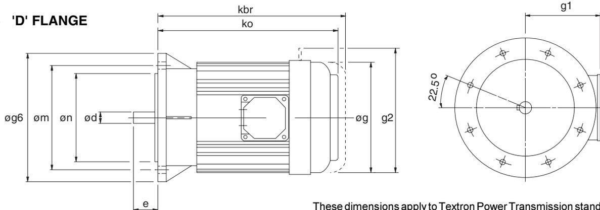
These dimensions apply to Textron Power Transmission standard motors
